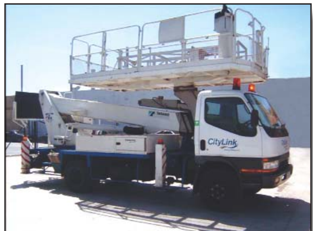
1999 Tadano AT150S 16.4M working height Super Deck with 800 kg deck capacity, 360 degrees continuous boom & deck swing. Mounted on a Mitsubishi Canter Carrier 5,641 Hours, 96,697 Klms As is condition, No 10 year test Price $115,000 + GST or 10 year tested $155,000 + GST, ex stock Adel.
